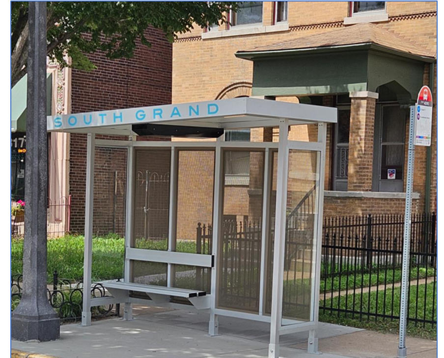
A MetroBus stop with a shelter featuring perforated metal walls, allowing for transparency and easier maintenance
